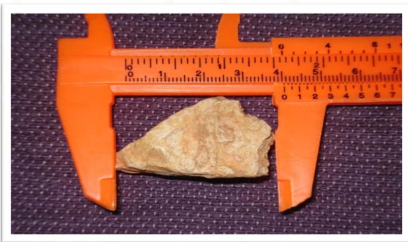
Figure 3.3. Measuring an object using a Vernier caliper.
